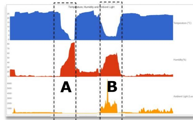
Figure 5. Time series plot of temperature, humidity, and ambient light sensor data. The section labelled A shows the outdoor data sample collected at dawn, and the section labelled B shows outdoor data collected in the morning
